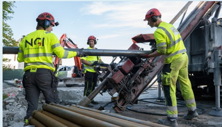
Extraction of soil cores by NGI to evaluate ground conditions before excavation and construction.
